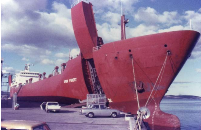
Top left: M/V Avon Forest, view of the starboard bow with shell doors open, Macquarie Wharf No. 2, Hobart, Tasmania, late 1979. Photograph by William Edward Burton, wburton@iinet.net.au .
