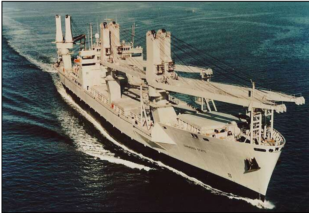
Figure 1: Crane ship Diamond State with heavy-lift cranes mounted in pairs on the Main Deck. Maritime Administration photograph, from Diamond State historical information. 1
