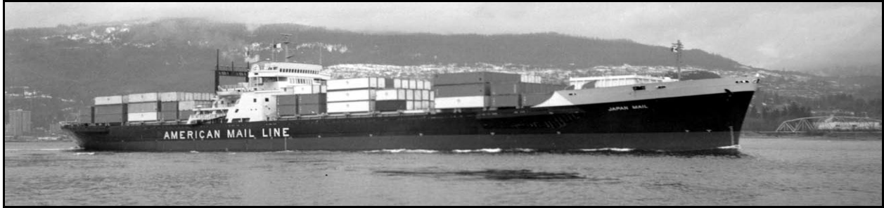
Figure 3: The Japan Mail at Vancouver, British Columbia, January 23, 1972, after being lengthened and converted to all-containerized cargo. 8
