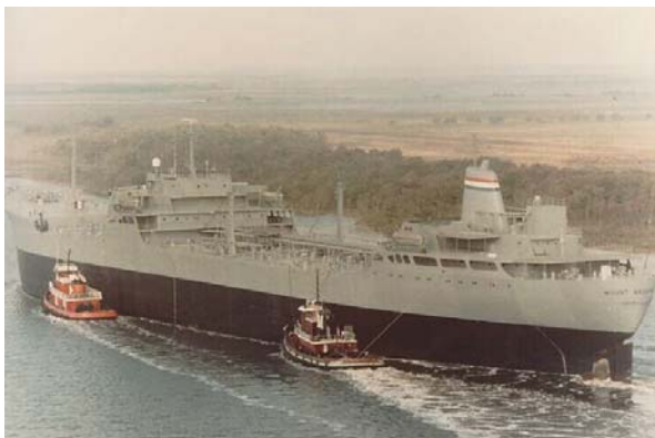
Left: The Mount Washington , built in 1963, with the traditional divided superstructure. Right: Mission Buenaventura , designed with an all-aft superstructure. Maritime Administration photos.
