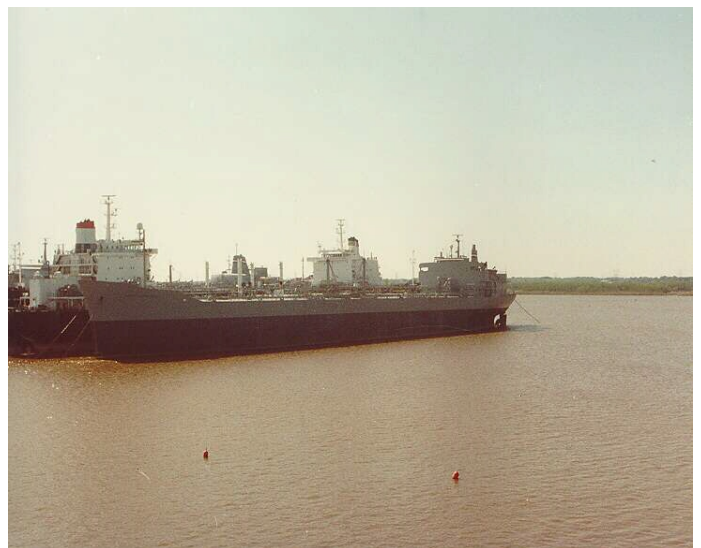
Left: The Mount Washington , built in 1963, with the traditional divided superstructure. Right: Mission Buenaventura , designed with an all-aft superstructure. Maritime Administration photos.
