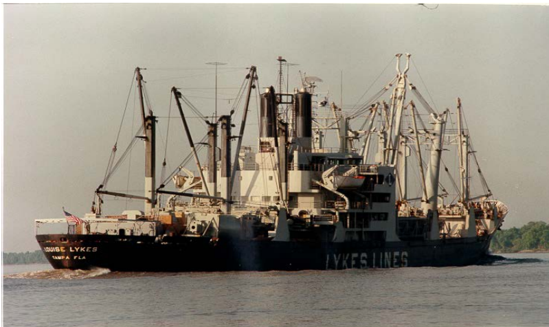
Bottom: Louise Lykes circa 1960s. Note the kingpost & booms with the heavy lift boom forward, raised forecandle and superstructure (with machinery below) at the 2/3 aft position. Maritime Administration photographs.
