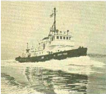
Foss Launch and Tug Co. tugboat HENRY FOSS is powered by a pair of 8 cylinder Series 13 inline engines providing a total of 5000 hp. These engines, OPERATING ON INEXPENSIVE BLENDED FUEL OIL, deliver the sort of smooth, reliable performance usually associated only with lighter fuels.
