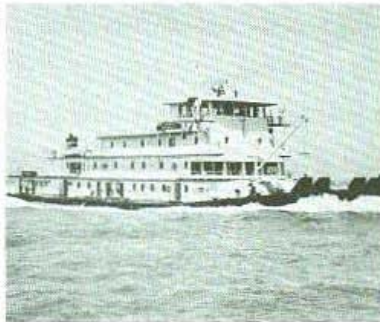
Propulsion power aboard the M/V MISSISSIPPI, 271 foot U.S. Corps of Engineers towboat, is furnished by a pair of 1860 hp Series 13 inline diesels.
