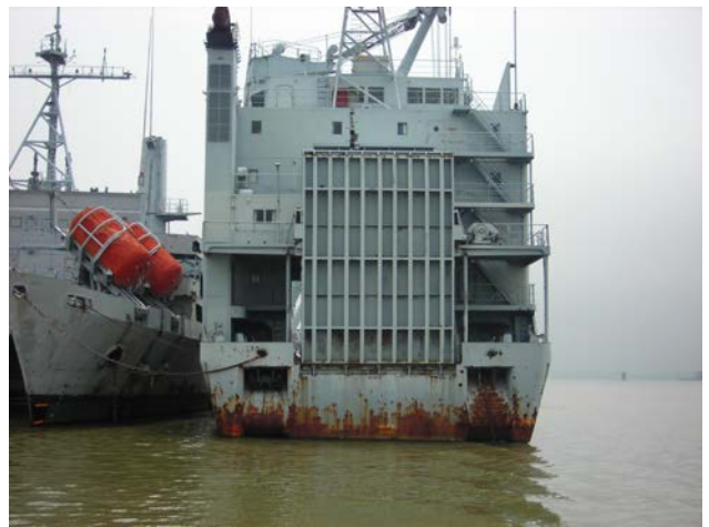
Clockwise from top left: Stern ramp closed aft of the ship's superstructure; Heavy lift boom near the ship's bow; Stern ramp closed; Heavy lift boom; Ship's bow, which also opens on either side to access the bow ramp. Maritime Administration photographs.
