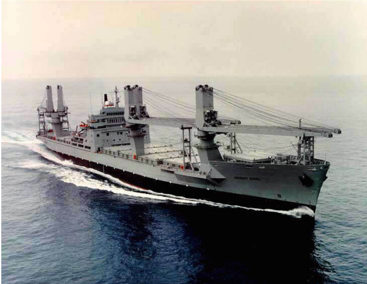
Aerial view of Equality State underway showing its heavy-lift cranes mounted in pairs on the Main Deck. Maritime Administration photograph.
