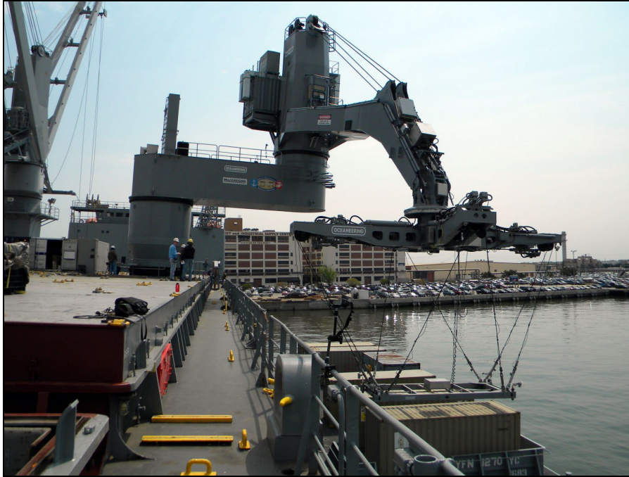
Figure 5: Large Vessel Interface Lift-on/Lift-off (LVI Lo/Lo) crane at Naval Station Norfolk, 14 April 2010, temporarily installed on SS Flickertail State (ACS 5), uses motion-sensing technology .Alongside SS Flickertail State is the open/covered lighter YFN-1270. (U.S. Navy Photo) 14
